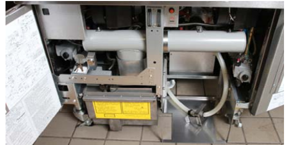
Figure 1: The fryer prior to the install is show above. The sensor mounts on the channel behind the center upright. The pre-filter mounts above the filter pan pickup .
